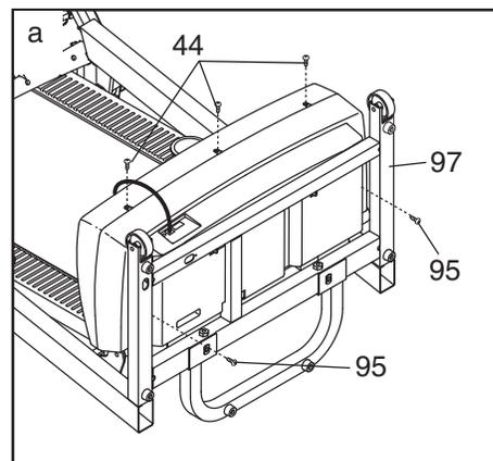
With the help of a second person, carefully raise the Uprights (97) as shown. Carefully pivot the Hood (93) off.
