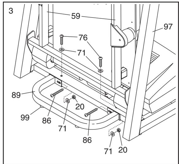
4. Lower the treadmill Frame (59) (see HOW TO LOWER THE TREADMILL FOR USE on page 21). With the help of a second person, carefully tip the Uprights (97) down as shown.
