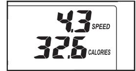
If one of the numbered speed buttons is pressed, the walking belt will gradually increase in speed until it reaches the selected speed setting.
