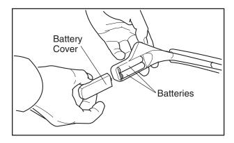
Note the markings inside the battery compartment showing which direction batteries must be turned. Insert two "AAA" batteries into the battery compartment. Replace the battery cover.
