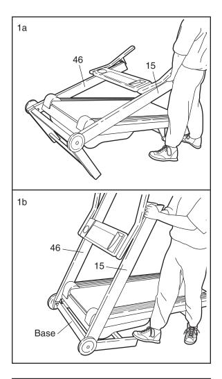
2. Pivot the Console (17) upward until it stops. Using the included allen wrench, tighten a 3/8" x 1 1/4" Bolt (45) into each Upright (15, 46).
