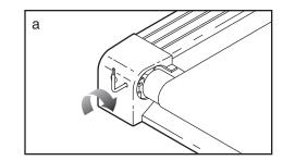
b. If the walking belt has shifted to the right, first remove the KEY and UNPLUG THE POWER CORD. Using the 3/16" end of the allen wrench, turn the left rear roller adjustment bolt counterclockwise 1/4 of a turn. Plug in the power cord, insert the KEY and run the treadmill for a few minutes. Repeat until the walking belt is centered.
