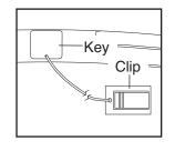
gency, the key can be pulled from the console, causing the walking belt to slow to a stop. Test the clip by carefully taking a few steps backward; if the key is not pulled from the console, adjust the position of the clip.
