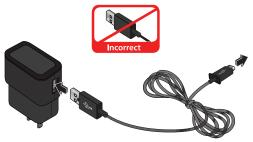
Plug the charging head into a standard AC power outlet. The device turns on with the screen locked and indicates both its charge state and percent of charge.
