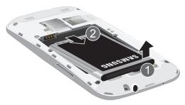
3. Lift the battery up and out of the phone (2).
