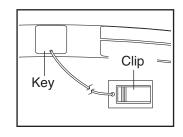
the console. After several seconds, the displays will light. IMPORTANT: In an emergency, the key can be pulled from the console, causing the walking belt to slow to a stop. Test the clip by carefully taking a few steps backward; if the key is not pulled from the console, adjust the position of the clip.
