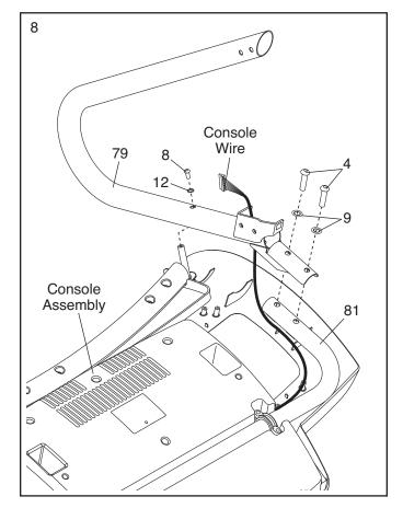
With the help of a second person, grip the sides of the console assembly and hold it near the Right Upright (83) and the Left Upright (not shown). Do not lift the console assembly by the Right Handrail (79) or the Left Handrail (not shown).
