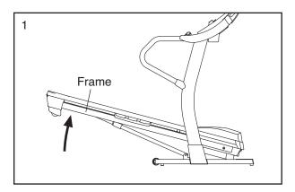
Raise the frame until the latch knob locks in the storage position. CAUTION: Make sure that the latch knob locks.
