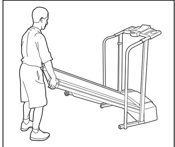
2. Move your right hand to the position shown and hold the treadmill firmly. Raise the treadmill until the storage latch closes over the catch. **Make sure that the storage latch is fully engaged over the catch.**
