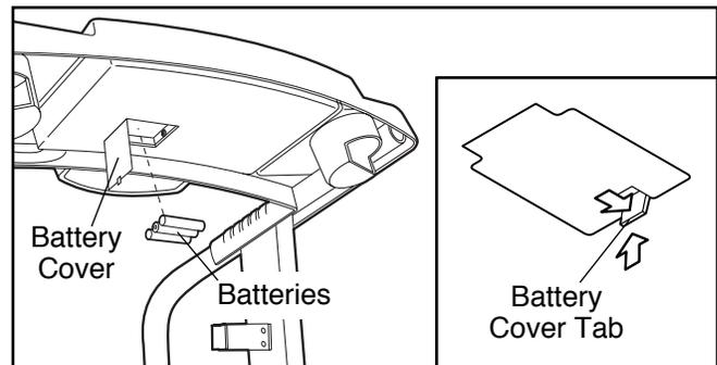
batteries are touching the springs in the battery compartment. Close the battery cover, push up on the battery cover tab, and then push the tab forward as shown in the inset drawing. Be sure that the tab locks into place.
