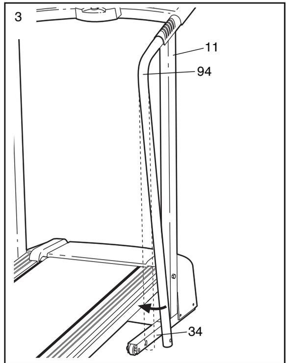
4. Attach the Right Handrail (94) to the Extension Leg (34) with a Handrail Bolt (93), a Handrail Washer (92) and a Handrail Nut (91).
