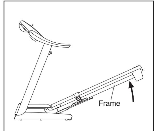
2. Move your right hand to the position shown and hold the treadmill firmly. Using your left hand, pull the latch knob to the left and hold it. Raise the frame until the catch is past the latch pin. Slowly release the latch knob. **Make sure that the catch is securely held by the latch pin.**
