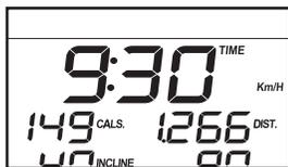
Note: The console can display speed and distance in either miles or kilometers. A "Km/H" will appear in the right side of the display when the console is displaying speed and distance in kilometers. To change the unit of measurement, see THE INFORMATION MODE on page 19. **Note: For simplicity, all instructions in this section refer to miles.**
