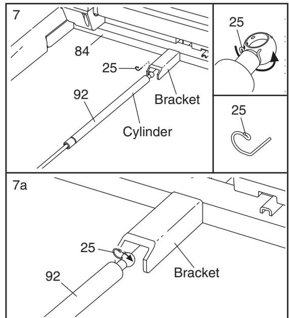
8. Raise the Gas Spring (92) to a vertical position. Remove the Spring Pin (25) from the raised end of the Gas Spring as described in step 7. If necessary, rotate the Gas Spring to align the end of the Gas Spring with the ball on the bracket on the Frame (58).
