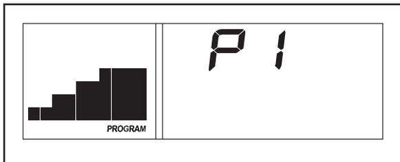
A few seconds after a personal trainer program is selected, the maximum incline setting of the program and the maximum speed setting of the program will flash in the display for a few seconds. The display will then show how long the program will last. A profile of the speed settings of the program will scroll across the matrix.
