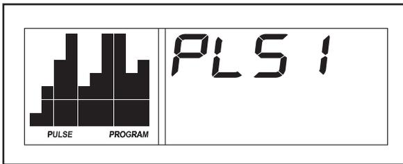
If pulse program 1 is selected, a profile of the target heart rate settings of the program will scroll across the matrix.
