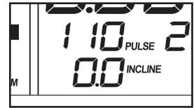
If pulse program 10 is selected, the maximum target heart rate setting of the program will flash in the display. If desired, press the Heart Rate increase and decrease buttons to change the maximum target heart rate setting (see EXERCISE INTENSITY on page 24). Note: If the maximum target heart rate setting is changed, the intensity level of the entire program will change.
