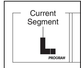
When the first segment of the program ends, a series of tones will sound and the current speed setting and the current incline setting will be saved in memory. *The three columns of indicators will then move one column to the left*, and the speed setting for the second segment will be shown in the flashing Current Segment column. Program a speed setting and an incline setting for the second segment as described above.
