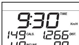
Note: The console can display speed and distance in either miles or kilometers. A "Km/H" will appear in the right side of the display when the console is displaying speed and distance in kilometers. To change the unit of measurement, see THE INFORMATION MODE/DEMO MODE on page 19. **Note: For simplicity, all instructions in this section refer to miles.**
