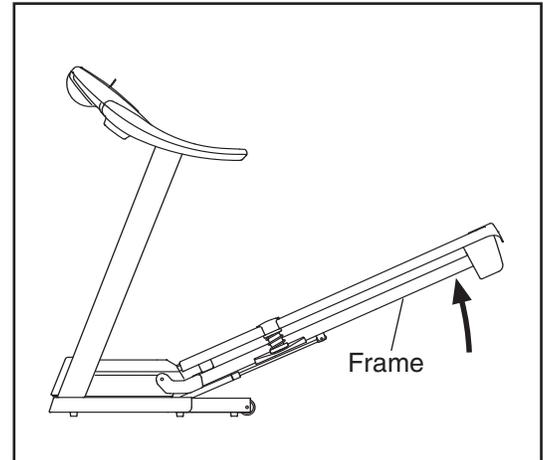
2. Move your right hand to the position shown and hold the treadmill firmly. Using your left hand, pull the latch knob to the left and hold it. Raise the treadmill until the catch is past the latch pin. Slowly release the latch knob. **Make sure that the catch is securely held by the latch pin.**
