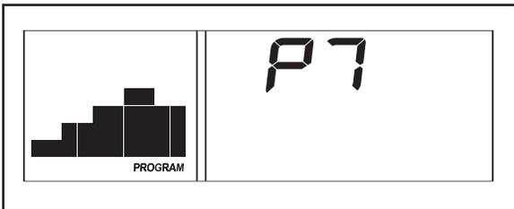
A few seconds after a custom program is selected, the maximum incline setting of the program and the maximum speed setting of the program will flash in the display for a few seconds. The display will also show how long the program will last. A profile of the speed settings of the program will scroll across the matrix.
