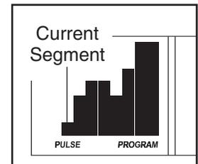
When the first segment ends, *all target heart rate settings will move one column to the left*. The target heart rate setting for the second segment will then be shown in the flashing Current Segment column.
