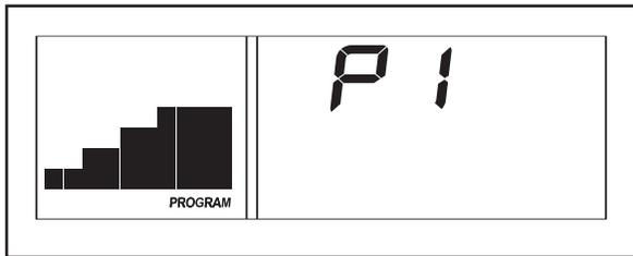
A few seconds after a personal trainer program is selected, the maximum incline setting of the program and the maximum speed setting of the program will flash in the display for a few seconds. The display will also show how long the program will last. A profile of the speed settings of the program will scroll across the matrix.
