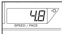
$\nabla$  button. A number will begin to flash in the SPEED/PACE display. This number is the maximum speed that the treadmill will reach during the program. Press the SPEED  $\Delta$  or  $\nabla$  button repeatedly to change the maximum speed setting. If the setting is increased, the difficulty level of the entire program will increase; if the setting is decreased, the difficulty level of the entire program will decrease.
