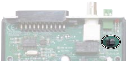
fig.3: moving the jumpers (12V output or N.O. contact)
