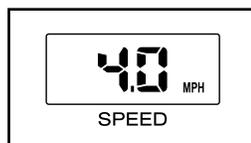
Note: The console can display speed and distance in either miles or kilometers. The letters MPH or KPH in the Speed display will show which unit of measurement is selected. To change the unit of measurement, hold down the Stop button, insert the key into the console, and continue to hold the Stop button for a moment. An “E” for English miles or an “M” for metric kilometers will appear in the Fat Calories/Calories display. Press the Speed  $\Delta$  button to change the unit of mea-
