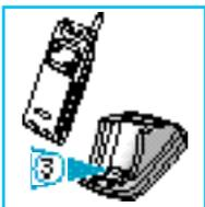
3. If you do not wish to use your phone while charging the battery, you can leave the battery attached to the phone. Place the phone with the battery attached in the front compartment of the charger with the keypad facing forward.
