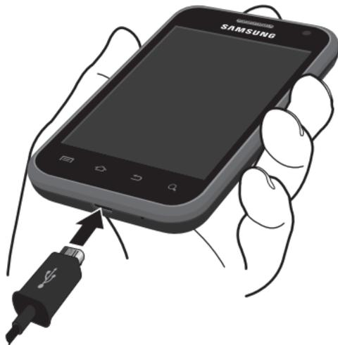
3. Insert the USB cable into the port (2).
