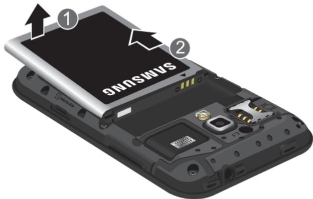
3. Lift the battery up and out of the phone (2).
