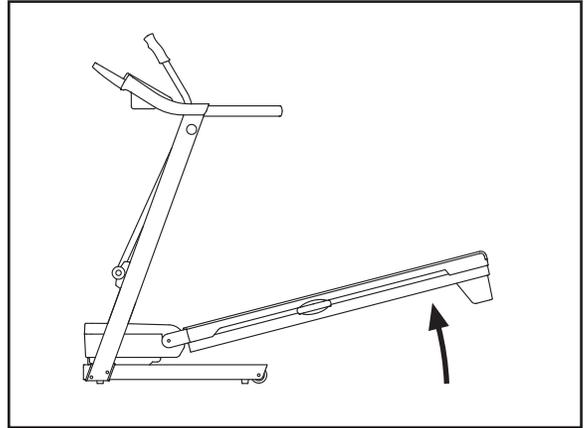
2. Move your right hand to the position shown and hold the treadmill firmly. Using your left hand, pull the latch knob to the left and hold it. Raise the frame until the pin is aligned with the gap between the frame and platform, and then slowly release the latch knob. **Make sure that the latch pin is fully inserted into the gap.**
