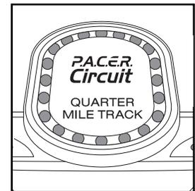
**Time display**—When the manual mode or the iFIT.com mode is selected, this display will show the elapsed time. When a workout program is selected, the display will show the time remaining in the program and the time remaining in the current segment of the program. The display will alternate between one number and the other every few seconds, as shown by the indicators in the display.
