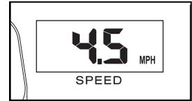
As you exercise, change the speed of the walking belt as desired by pressing the Speed buttons. Each time a button is pressed, the speed will change by 0.1 mph. If a button is held down, the speed will change in increments of 0.5 mph.
