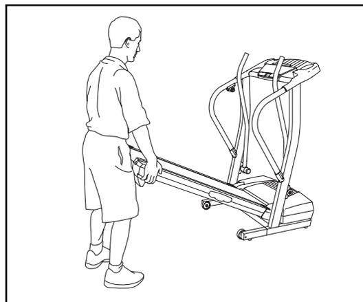
2. Move your right hand to the position shown and hold the treadmill firmly. Using your left hand, pull the latch knob to the left and hold it. Raise the treadmill until the frame is past the latch pin. Slowly release the latch knob. **Make sure that the frame is securely held by the latch pin.**
