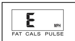
**Fat Calories/Calories/Pulse display**—This display shows the approximate numbers of *fat calories* and *calories* you have burned (see FAT BURNING on page 22). The display will alternate between one number and the other every few seconds, as shown by the indicators in the display. The display will also show your heart rate when you use the pulse sensor (see step 6).
