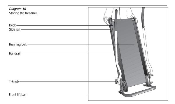
To store the treadmill in a vertical position as shown in Diagram 16 and free up floor space when the treadmill is not in use, take the following steps:
