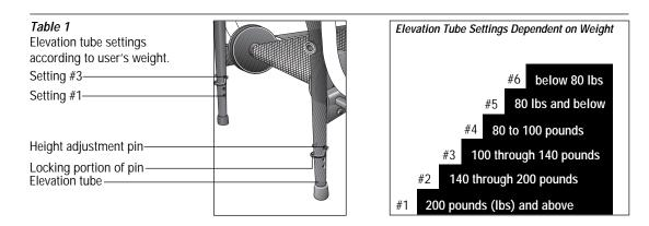
Table 1 is an approximation and elevation tube settings may vary slightly depending on differences in weight and the amount of lubrication between the running belt and deck. Over time and extended use, you may need to readjust the elevation tube setting or add lubricant between the running belt and deck—this is normal and does not require a service call.
