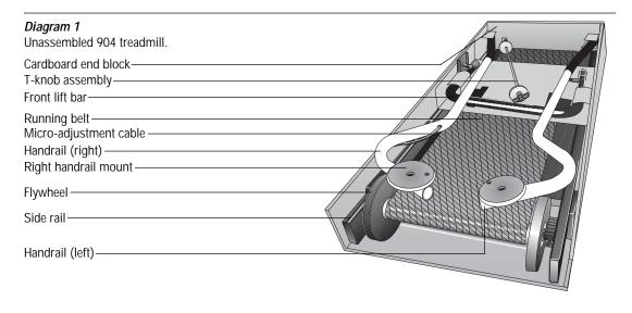
Diagram 1 shows the treadmill's parts after opening the carton. Callouts point to the different parts of the treadmill that are discussed in the assembly instructions. Unpack the treadmill close to the location where you plan to use it.
