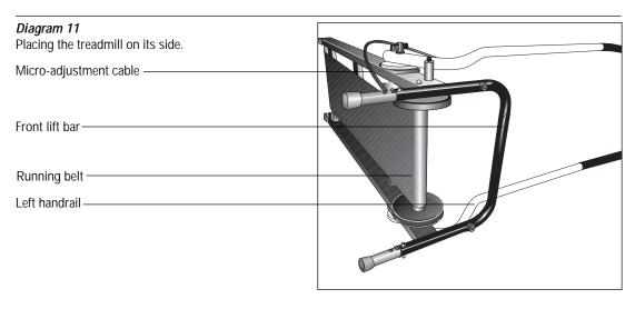
*CAUTION: Be sure that the T-knobs are secure and the handrails are locked into position on both sides before performing this step.*Position the Treadmill on Its Side. (Diagram 11) Place one hand on each handrail and gently tip the treadmill onto its side opposite the micro-adjustment knob. See Diagram 11. Be sure the treadmill is balanced and secure on its side and the micro-adjustment knob is *not* resting on the floor, before you let go of the handrails.
