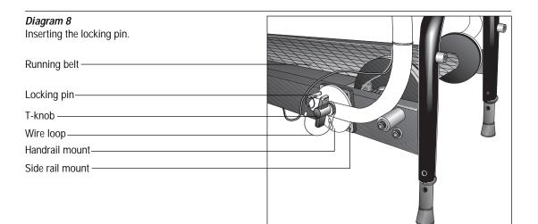
e. Remove the locking pin (D) from the hardware kit and place the wire loop over the T-knob. Align the hole in the handrail mount with the side rail mount and insert the locking pin. See Diagram 8.
