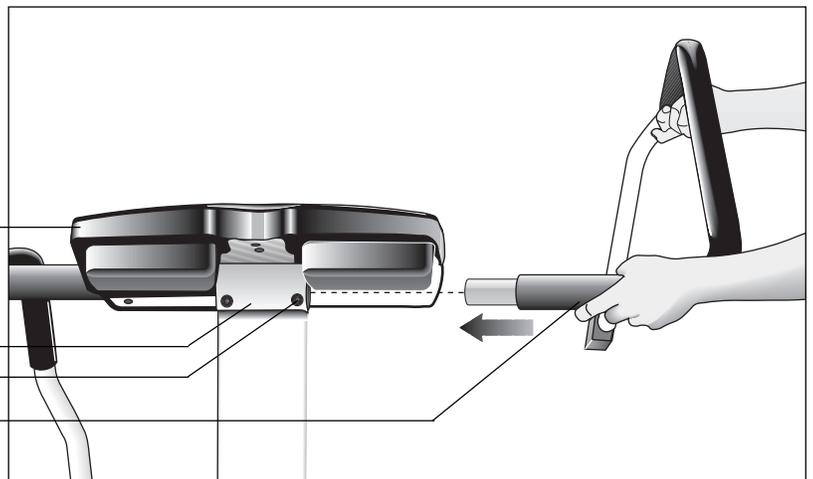
9. Insert the upper end of a handrail into the upper handrail clamp. Using one hand, apply pressure on the portion of the handrail going into the clamp while, with the other hand, lift and lower the base of the handrail. This rotating motion helps move the handrail into place. The handrail is properly positioned when the black foam wrap touches the clamp as shown in Diagram 5. Repeat this step for the other handrail.
