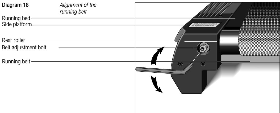
2. Locate the left belt adjustment bolt at the rear of the treadmill as shown in Diagram 18. The direction you turn the bolt depends on how the belt is tracking. Make all belt adjustments on the left rear corner bolt using the hex key provided.
