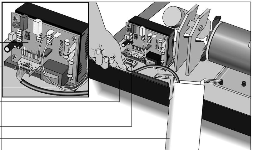
3. Set the upright column support assembly on the front plate. Route the ribbon cable under the lower board's cables. See inset in Diagram 3.
