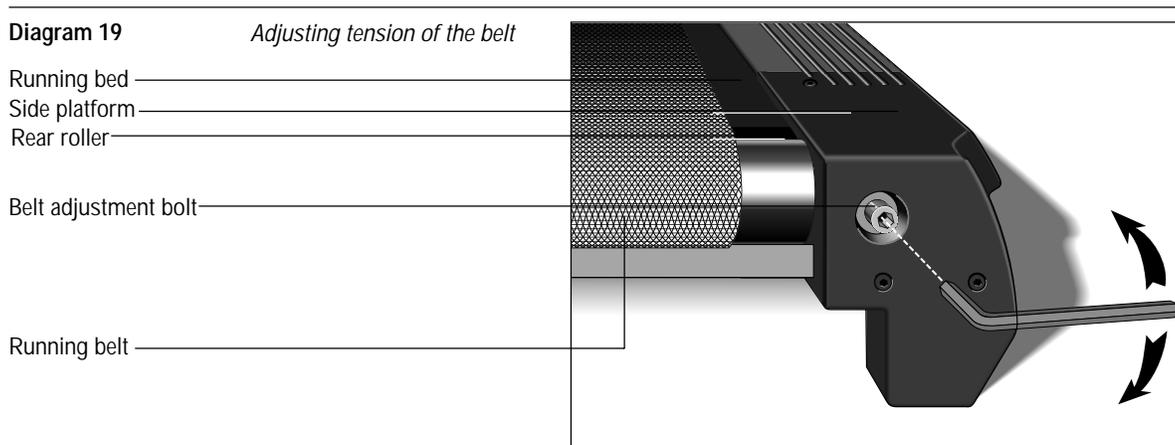
2. Standing behind the treadmill use the rear belt adjustment bolts (refer to Diagram 18 on the previous page and Diagram 19). Simply turn each bolt *clockwise* 1/4 turn to adjust the tension of the belt.
