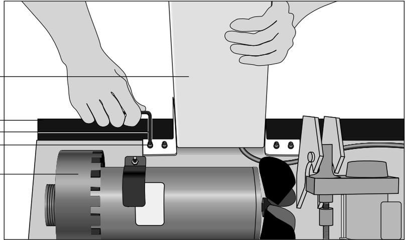
6. Secure the upright column support to the base by lifting it into position onto the base mounting plate. See Diagram 4. Align the bolt holes and hold onto the upright column support as you insert the frame-to-base bolts and finger tighten. Alternately tighten each bolt using the 5/16" hex key (F) provided.
