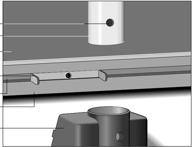
10. To mount the lower portion of the handrails, take the lower handrail clamps (J), two of the internal star washers (E), and lower handrail clamp bolts (C) out of the hardware kit. Refer to Diagram 6 while taking the following steps:
