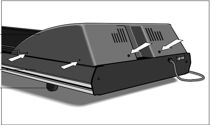
2. Remove the treadmill's hood using a phillips head screwdriver. Unscrew all six screws and set them aside. See Diagram 2. Grasp both sides of the hood with your hands and pull up to remove the hood from the base.
