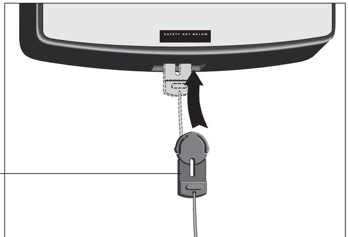
Before you can begin a workout, you must insert the magnetic safety key into the electronic console as shown in Diagram 9. The treadmill's running belt will not move unless the safety key is inserted and secure inside the electronic console. To prevent unauthorized use of the treadmill, store the safety key in a safe place.
