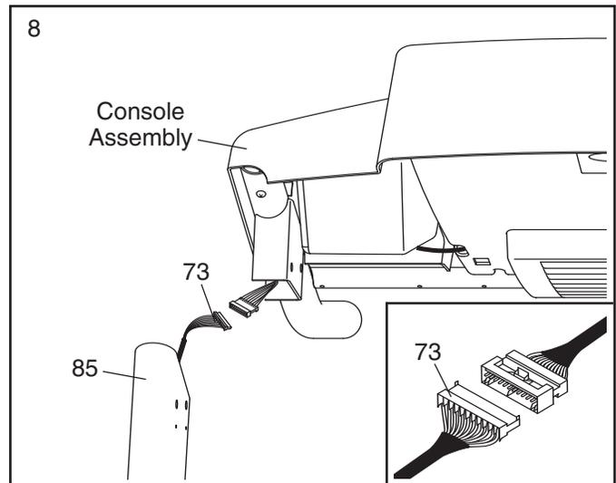
9. Remove the band securing the TV Cable (112) to the left Upright (85). Connect the TV Cable to the cable extending from the console assembly. Then, insert the TV Cable into the left Upright.
