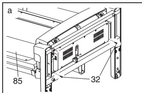
Raise the Uprights (85) to the vertical position. Remove the three 3/4" Screws (7) from the Hood (33), and carefully pivot the Hood off.
