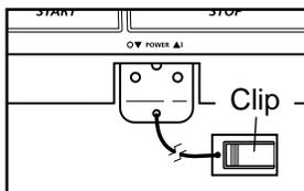
console. **Test the clip by carefully taking a few steps backward until the key is pulled from the console. If the key is not pulled from the console, adjust the position of the clip as needed.** Then, remove the key from the console.
