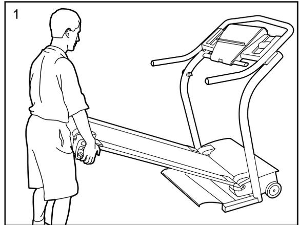
2. Move your right hand to the position shown and hold the treadmill firmly. Using your left hand, pull the lock knob to the left and hold it. Raise the treadmill until the lock pin is aligned with the catch plate. **Make sure that the pin is resting on the plate as shown.**
