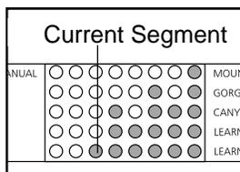
cline settings are not shown in the program display.) To program the desired speed and incline settings for the first segment, simply adjust the speed and incline of the treadmill to the desired levels with the Speed and Incline buttons. Every few times one of the Speed buttons is pressed, an additional indicator will light or darken in the Current Segment column.
