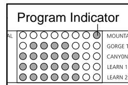
When you select a preset program, the program display will show a simplified profile of the program you have selected. For example, the profile above shows that the intensity of the selected program will be greater during the middle of the program and less during the beginning and end. The Time/Laps display will show how long the program will last.
