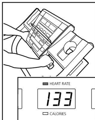
**moving your hands.** When your pulse is detected, the Heart Rate indicator will flash, three dashes (— — —) will appear in the Heart Rate/Calories display, and then your heart rate will be shown. **For the most accurate heart rate reading, continue to hold the contacts for about 15 seconds.**
