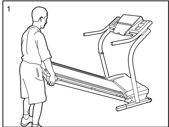
2. Move your right hand to the position shown and hold the treadmill firmly. Using your left hand, pull the latch knob to the left and hold it. Raise the treadmill until the pin on the lock knob is aligned with the hole in the catch. Insert the pin into the catch. **Make sure that the pin is fully inserted into the catch.**
