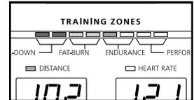
**Time/Laps display**—When the manual mode or an iFIT.com program is selected, this display will show the elapsed time and the number of 1/4-mile laps you have completed. When a preset program or a custom program is selected, the display will show the time remaining in the program, the time remaining in the current segment of the program, and the number of 1/4-mile laps you have completed. The display will change from one number to the next every seven seconds.
