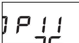
As each custom program is selected, the maximum speed setting of the program and the maximum incline setting of the program will flash in the displays for a few seconds. The Time/Distance display will show how long the program will last. A profile of the speed settings of the program will scroll across the matrix. **Note: If only three columns of indicators scroll across the matrix, see HOW TO CREATE A CUSTOM PROGRAM on page 16.**
