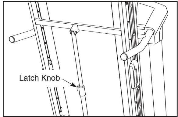
2. **Hold the metal frame firmly with both hands, and lower it to the floor. CAUTION: To decrease the possibility of injury, do not lower the frame by gripping only the plastic foot rails. Do not drop the frame to the floor. Make sure to bend your legs and keep your back straight.**
