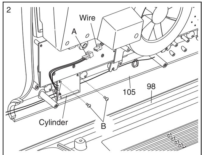
3. **Make sure that no wires are pinched.** See drawing 1. Reattach the Console (105) to the Console Base (98) with the Screws (99). Discard the other wires included with the receiver.
