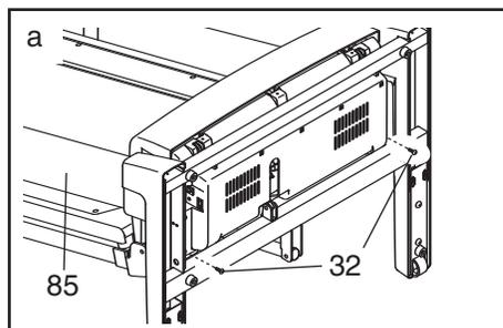
Raise the Upright (85) to the vertical position. Remove the three 3/4" Screws (7) from the Motor Hood (33), and carefully pivot the Motor Hood off.
