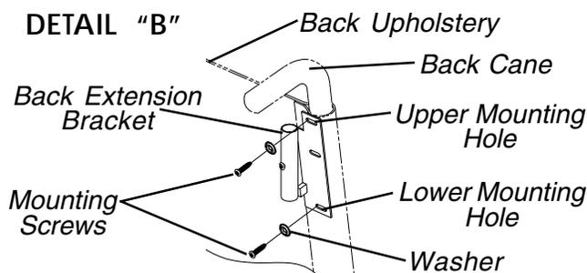
FIGURE 1 - INSTALLING THE BACK EXTENSION BRACKETS
