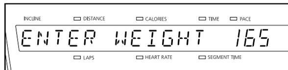
display. Press the Enter Weight buttons again to enter your weight. The buttons can be held down to enter your weight quickly. Four seconds after the buttons are last pressed, the weight setting will disappear from the display. Your weight will then be saved in memory.
