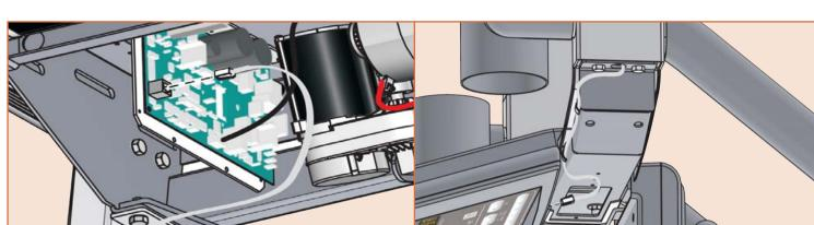
Hardware Needed over tighten them. Tighten the screws securely but do not covers before tightening the screws. to align the edges of the top and bottom to the bridge/console assembly. Be sure from the bottom, secure the bridge cover the top and (4) #6 x 3/8 Phillips screws Using (2) #10 x 1/2" Phillips screws from
