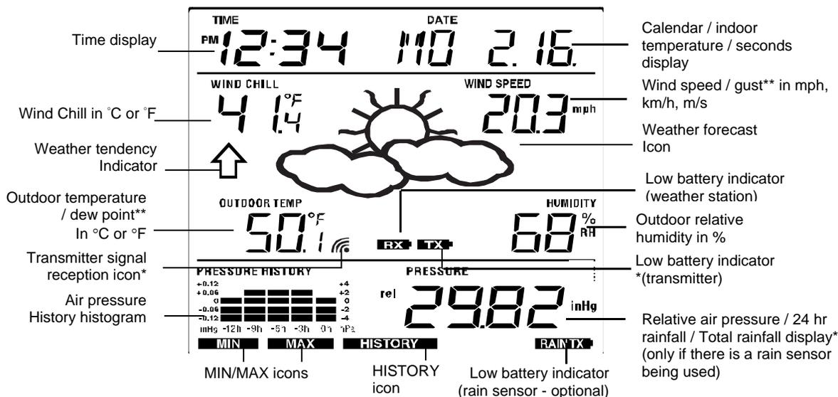
\* When the signal from the transmitter/ or rain sensor (optional) is successfully received by the Weather Station, this icon will be switched on. (If not successful, the icon will not be shown on the LCD). User can therefore easily see whether the last reception was successful ("ON" icon) or not ("OFF" icon). On the other hand, the short blinking of the icon shows that a reception is being done at that time.
