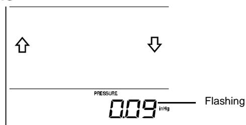
You may select a definite switching sensitivity value, .06, .09, or .12 inHg (2-4 hPa) for the change in the display of weather icons. This represents the "sensitivity" of the weather forecast (the smaller the value selected, the more sensitive the weather forecast). The default value is 0.09 inHg (3 hPa).
