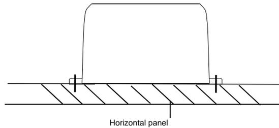
For best results, the rain sensor should be securely mounted onto a horizontal surface about 39.37" (1 meter) above the ground (or higher) and in an open area away from trees or other coverings where rainfall may be reduced causing inaccurate readings.
