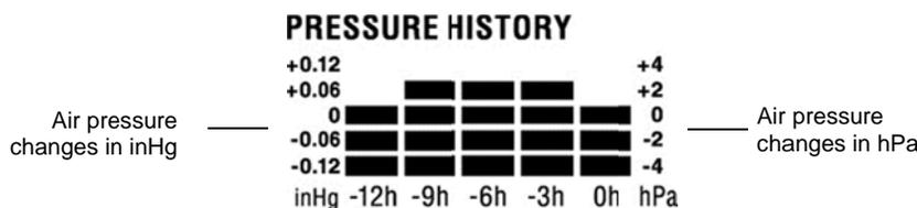
The horizontal axis represents the last 12 hours air pressure recording (-12, -9, -6, -3 and 0 hour). The bars are plotted at each of the 5 steps and give the trend over the recorded period. The scale on the right compares the result. The "0" in the middle of this scale determines the current air pressure.
