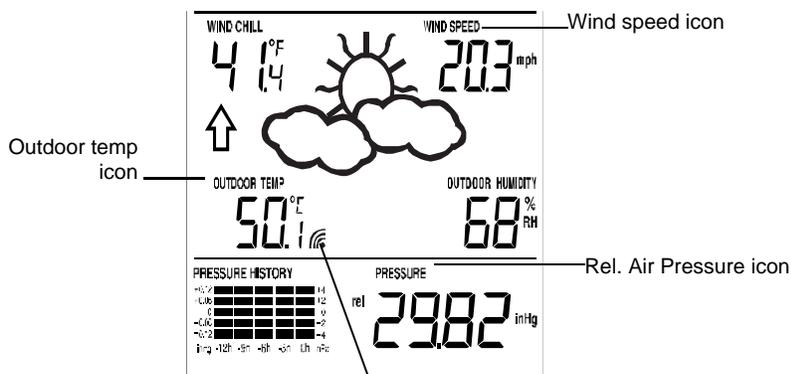
In Mode 1, this reception icon is showing the condition of the reception of the signal from Thermo-hygro transmitter
