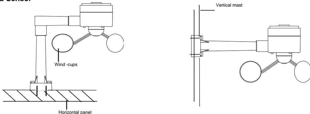
Check that the wind-cups can rotate freely before fixing the unit. For correct and accurate readings, it is important to mount the sensor with the cups on the bottom. The wind sensor should now be mounted using the screw or cable tie provided onto a solid wall/ panel mast or mast to allows the wind to travel around the sensor unhindered from all directions (ideal mast size should be from diameter 0.62" to 1.29" (16mm to 33mm). Do not over tighten the mounting bracket
