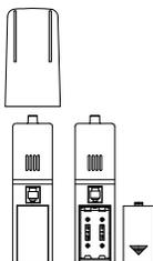
The outdoor Thermo-hygro transmitter works with 2 x AA IEC LR6, 1.5V batteries. To install and replace the batteries, please follow the steps below:
