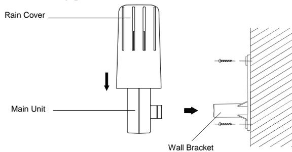
An ideal mounting place for the thermo-hygro sensor would be the outer wall beneath the extension of a roof, as this will protect the sensor from direct sunlight and other extreme weather conditions. Be sure to mount vertically.
