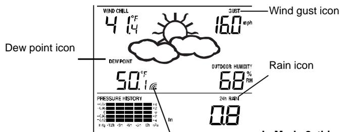
In Mode 2, this reception icon is showing the condition of the reception of the signal from Rain sensor (only if a rain sensor is being used).
