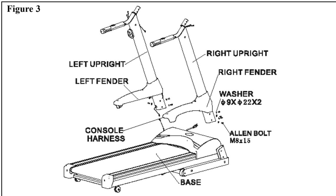
4. Attach the console assembly by connecting the console harness, incline harness, EKG harness, and speed harness as shown in Figure 4.
