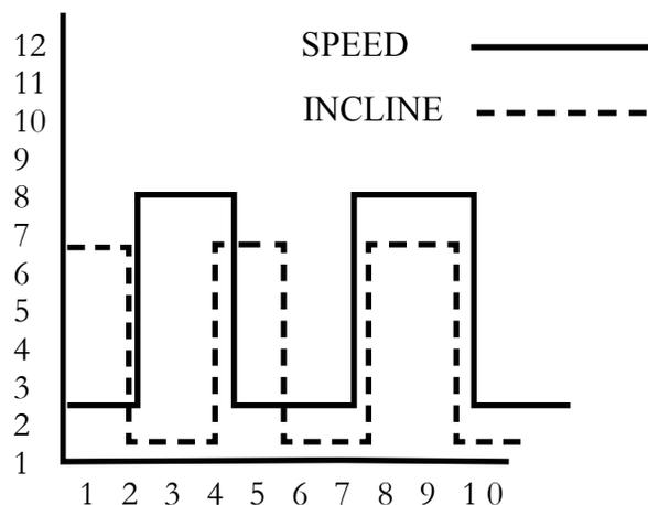
The **Cross Training Program** is designed to control the walking belt speed and elevation inversely in alternating segments.
