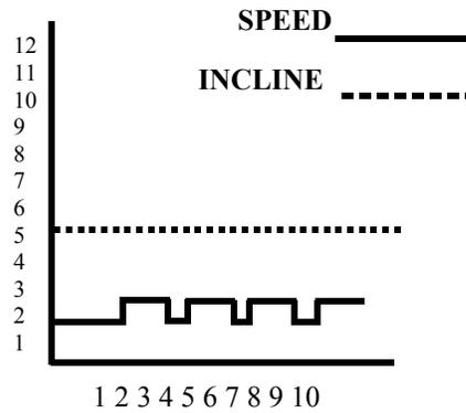
The **Cardio Program** is designed to vary the treadmill Speed, while maintaining a constant Elevation.
