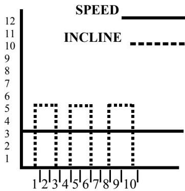
The **Fat Burn Program** is designed to vary the treadmill elevation, while maintaining a constant walking belt speed.
