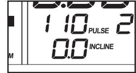
If pulse program 1, 3, or 4 is selected, the maximum target heart rate setting of the program will flash in the display. If desired, press the Incline increase and decrease buttons to change the maximum target heart rate setting (see EXERCISE INTENSITY on page 29). Note: If you change the maximum target heart rate setting, the intensity level of the entire program will change.
