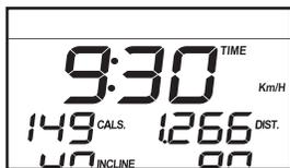
Note: The console can display speed and distance in either kilometers or miles. A "Km/H" will appear in the right side of the display when the console is displaying speed and distance in kilometers. To change the unit of measurement, see THE INFORMATION MODE on page 23. **Note: For simplicity, all instructions in this section refer to kilometers.**
