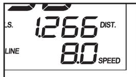
The center of the display is the priority display. Press the Display (DISP.) button repeatedly until the priority display shows the information that you most want to view. Note: While information is displayed in the priority display, the same information will not be displayed in the lower left or right corner of the display.
