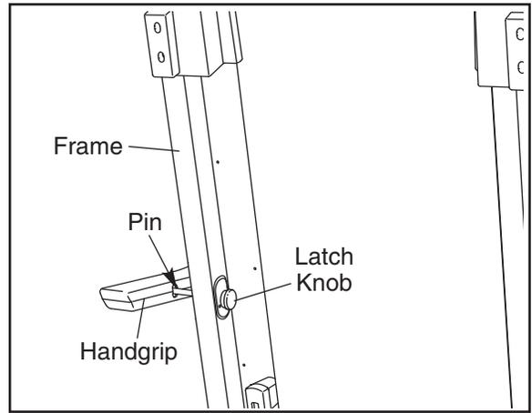
2. Hold the treadmill firmly with both hands, and lower the frame to the floor. **To decrease the possibility of injury, bend your legs and keep your back straight.**
