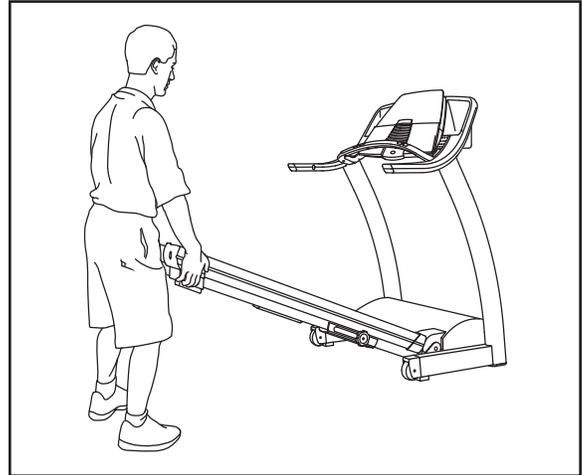
2. Hold the frame firmly with your left hand. Using your right hand, pull the latch knob to the right and hold it. Raise the frame until the pin on the latch knob is aligned with the hole in the left handgrip. Then, release the latch knob. **Make sure that the latch knob is fully released so that the pin is fully inserted into the hole in the left handgrip.**
