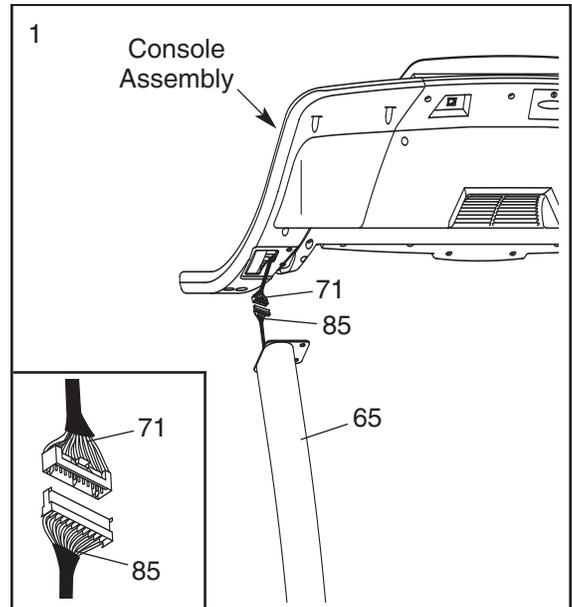
2. Insert the excess Wire Harnesses (71, 85) into the right Upright (65).
