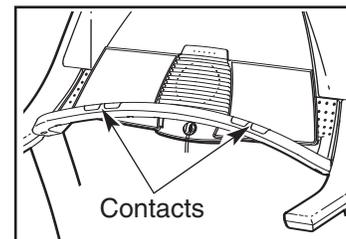
**Avoid moving your hands.** When your pulse is detected, two dashes (--) will appear in the Calories/Pulse display, and then your heart rate will be shown. **For the most accurate heart rate reading, continue to hold the contacts for about 15 seconds.**
