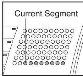
in the matrix.) To program a speed setting and an incline setting for the first segment, simply adjust the speed and incline of the treadmill as desired by pressing the Speed and Incline buttons. Every few times one of the Speed buttons is pressed, an additional indicator will light or darken in the Current Segment column.
