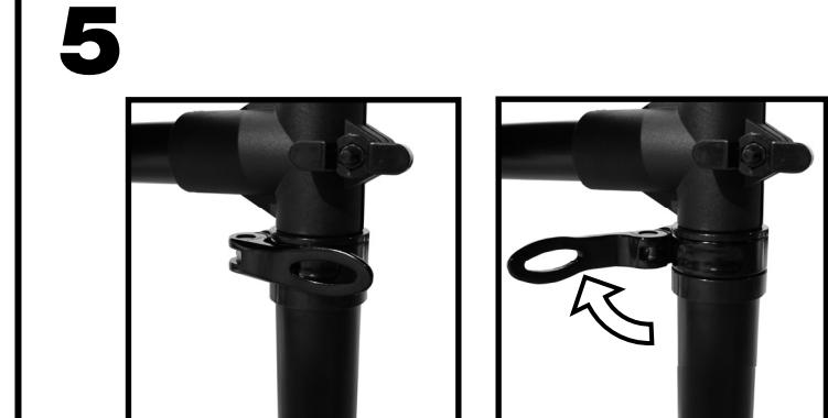
Open the four clamps near the tops of the rack legs, raise the upper part of the rack to an appropriate height, and close the clamps again to secure the rack in place. Make any other adjustments to the rack, drum pads, or cymbal pads/arms so all of the pads are within reach. See the **Connection Diagram** on the opposite page to connect the pads to the module.
