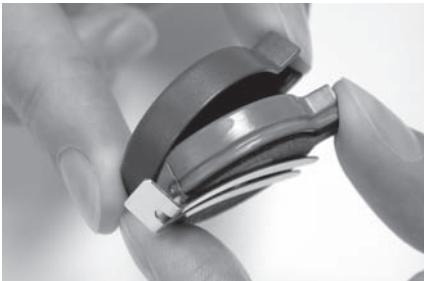
Figure 6: Fitting the Headpiece Color Cap.
