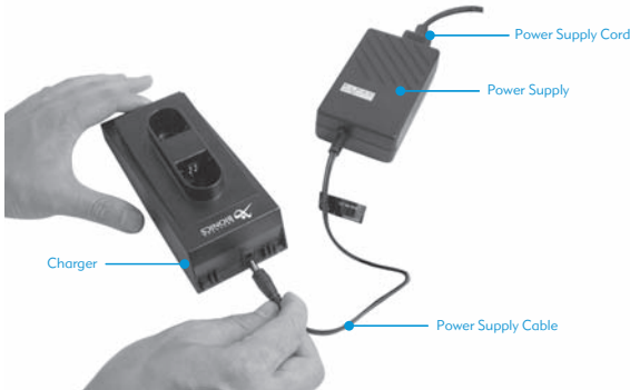
Figure 13: Connecting the Power Supply to the Charger.
