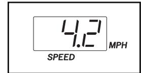
If one of the Quick Start buttons is pressed, the walking belt will gradually increase in speed until it reaches the selected speed setting. **Note: The console can display speed and distance in either miles or kilometres. For simplicity, all instructions in this section refer to miles.**
