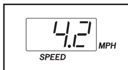
Note: The console can display speed and distance in either miles or kilometres. To find which unit of measurement is selected, hold down the Stop button while inserting the key into the console. An "E" for English miles or an "M" for metric kilometres will appear in the Speed display. Press the Speed increase button to change the unit of measurement. When the desired unit of measurement is selected, remove the key.
