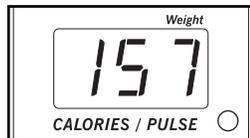
If you do not want to enter your weight, press the ENTER button. To enter your weight, press the SELECT buttons. Each time a button is pressed, the weight setting will change by 1 pound. If a button is held down, the weight setting will change in increments of 5 pounds. When the correct weight is shown, press the ENTER button. Once your weight is entered, it will be saved in memory.
