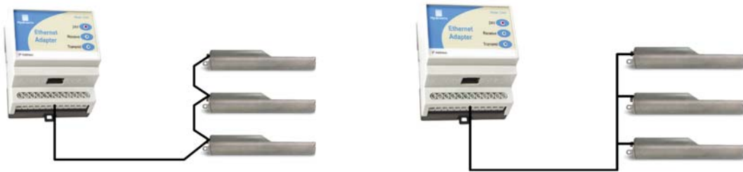
Figure 31: Redes de cables RS485 correctas
