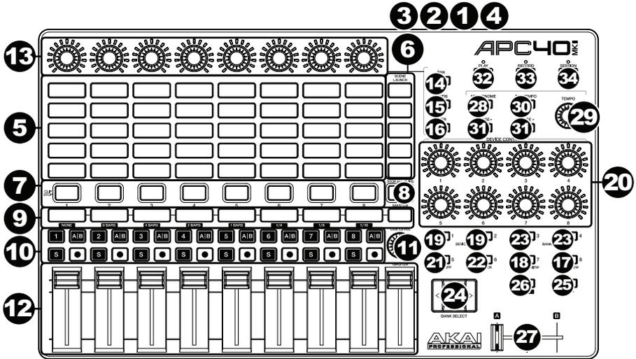
1. **USB Port:** Use a standard USB cable to connect this port to a USB port on your computer. The computer's USB port provides power to APC40 mkII. This connection is also used to send and receive MIDI data to and from your computer.
