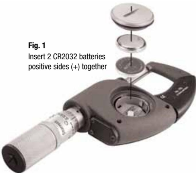
First, unscrew the battery cover from the back of the micrometer and install the **first battery with negative side down**. Next, install the second battery with the positive side down. Then, replace the cover making sure the rubber gasket is positioned correctly on the battery cover. The display will flash until the DATUM button is depressed to establish the DATUM position - see the section on "Setting the DATUM".
