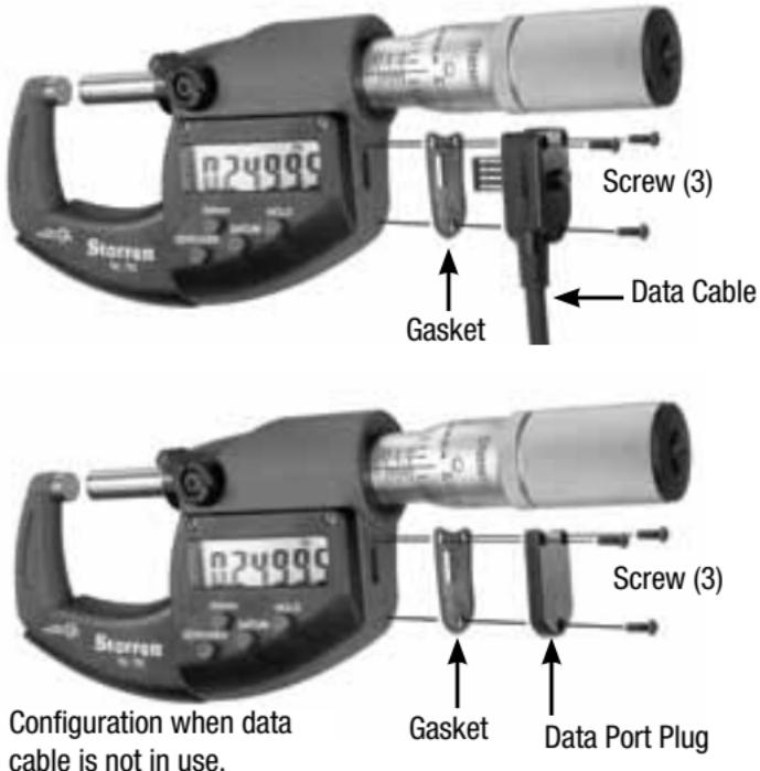
The output format is 4800 BAUD, 8 bits, No Parity, 2 stop bits ASCII data. Transmission is exactly 16 characters, followed by a carriage return and a line feed.
