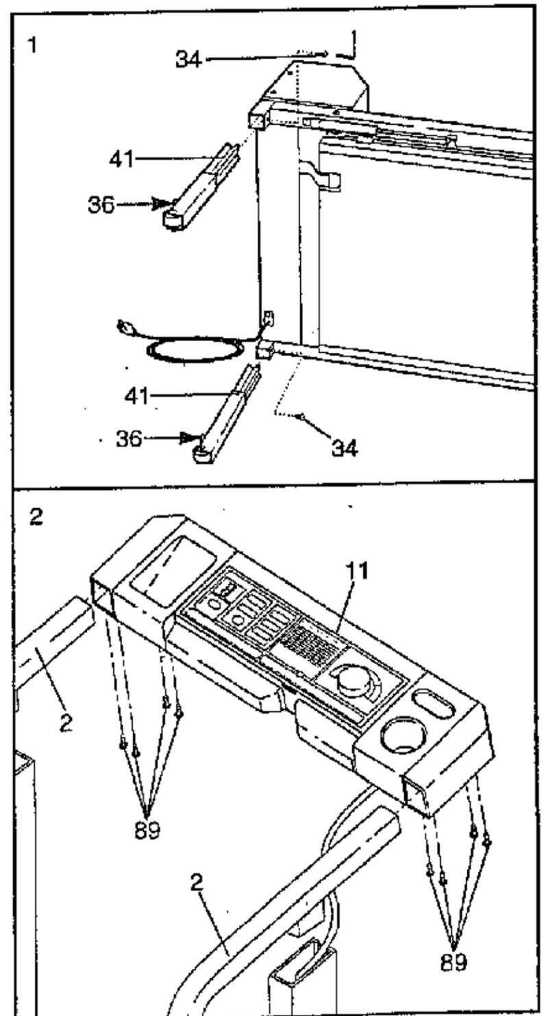
3. With the help of a second person, hold the Console (11) near the right Upright (14) as shown.
