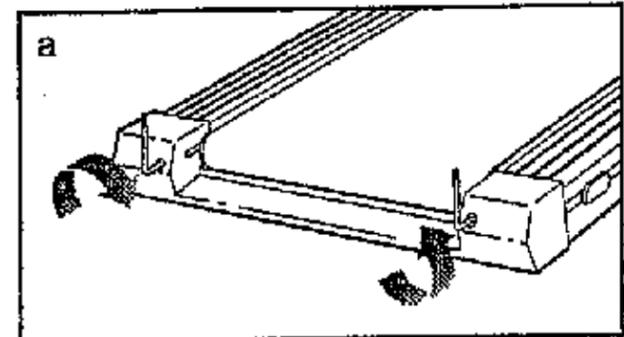
b. If the walking belt has shifted to the right, first remove the key and **UNPLUG THE POWER CORD**. Using the allen wrench, turn the left rear roller adjustment bolt counterclockwise, and the right bolt clockwise, 1/4 of a turn each. Be careful not to overtighten the walking belt. Plug in the power cord, insert the key and run the treadmill for a few minutes. Repeat until the walking belt is centered.
