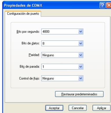
The computer is now correctly configured to receive data from the equipment. Press the **(Mem)** key and the **G-Test** will send all stored data to the computer, while the display shows the following message:
