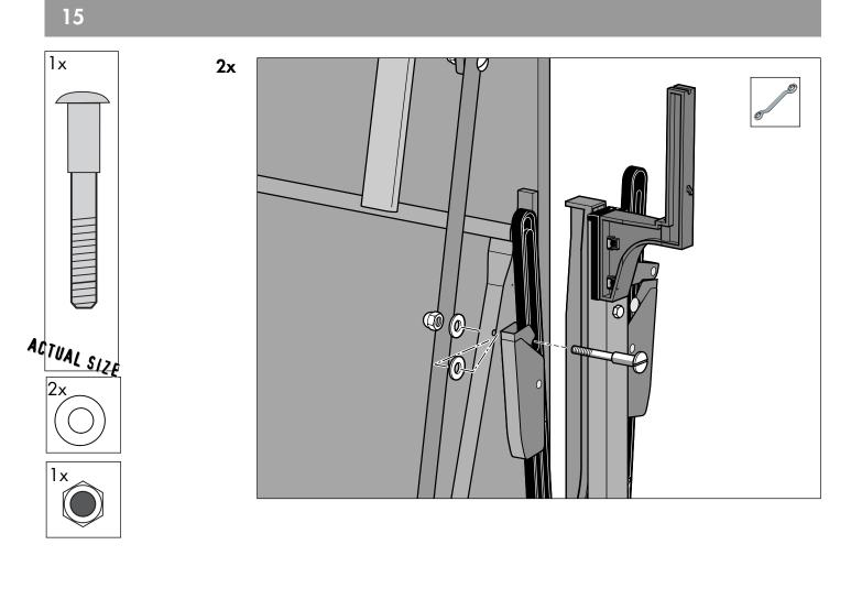
Carry out steps 12 – 15 for the second half of the table. Again, ensure that the table cannot slip or tilt over!
