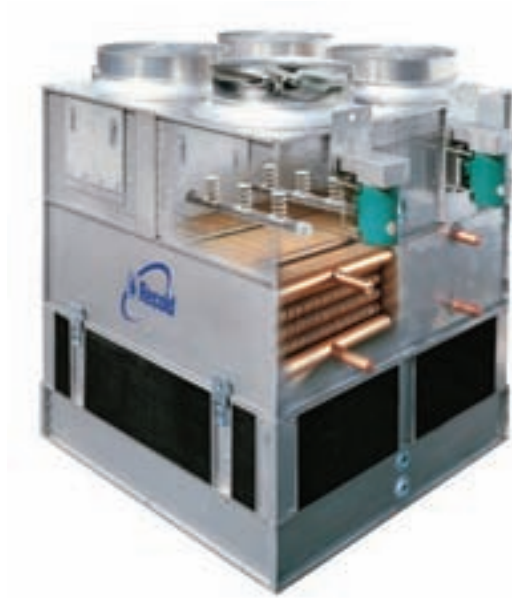
Recold MC Evaporative Condenser —Induced draft, counterflow design. G-235 galvanized steel factory assembled structure. Also available in 300 series stainless steel. Proven copper coil technology.
