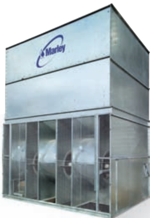
Marley Aquatower® Cooling Tower —Reliable performance has made this design the industry standard for more than 50 years. G-235 galvanized steel factory assembled structure. Also available in 300 series stainless steel. Capacities from 8 to 126 tons per cell. CTI Certified and FM Approved.
