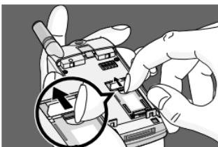
4. Close the SIM card holder, and move the holder lock lever up.
