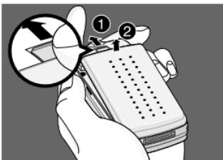
1. Unlock the battery cover ① and lift it off ②.
