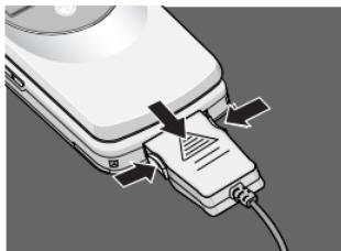
Disconnect the travel adapter from the phone by pressing its side buttons.
