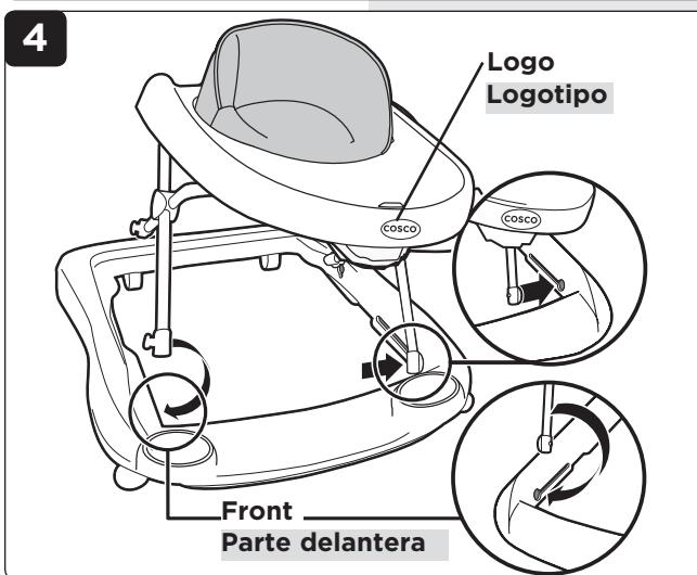
Orient the front of the tray to the front of the base as shown. Insert the post of one front leg into the track at the front of the base as shown in (**Figure 4**). Repeat with other front leg post, using gentle pressure to guide it into the track if necessary.
