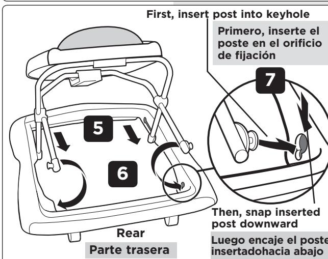
Align rear leg posts over the keyholes in rear of base as shown in (**Figure 6**). Using gentle pressure, squeeze the legs together to allow the posts to position into top of the keyholes.
