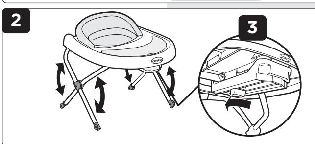
Pull down and twist height adjustment button counter-clockwise to lock legs in fully extended position as shown in (**Figure 3**).
