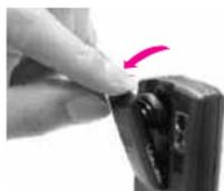
Simply press the release latch on the top of the phone, then pull the Bluetooth Headset to detach from the phone.
