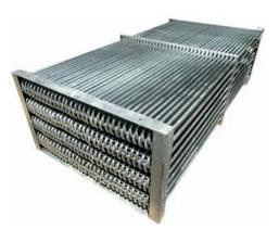
and welded into an assembly. The complete assembly is then hot-dip galvanized after fabrication. Design pressure is 1551 kPa, and each coil is tested to 2757 kPa air pressure under water. Tubes are sloped to provide free drainage when vented.
