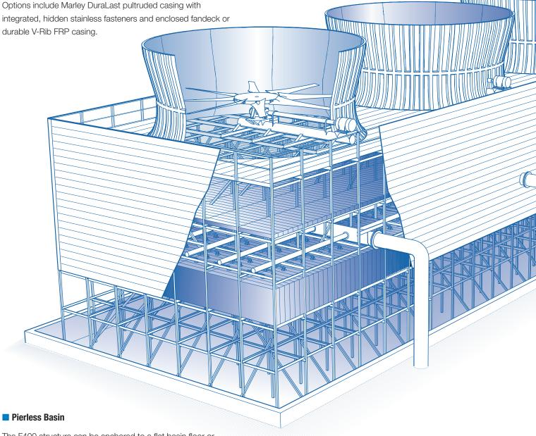
The F400 structure can be anchored to a flat basin floor or designed to fit existing basins. Fewer piers mean lower basin cost.
