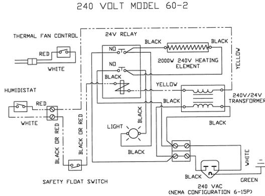
Figure 6 - Wiring diagram for Model 60-2 and F60-2 (240 volt) Steam Humidifier.
