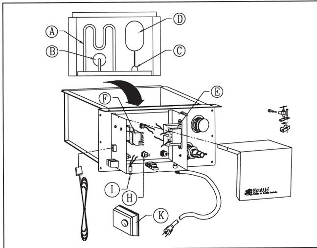
Figure 11 - Parts Diagram of Models 60-1, F60-1, 60-2 and F60-2
