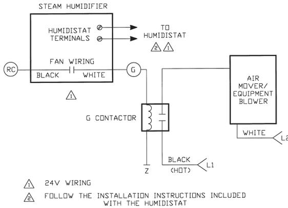
Figure 8B - Typical wiring for a humidifier in a single-speed air mover application without air conditioning (switching through a G contactor).
