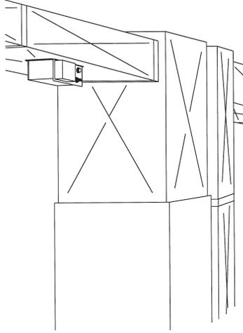
Figure 3 – Duct Center Mount
