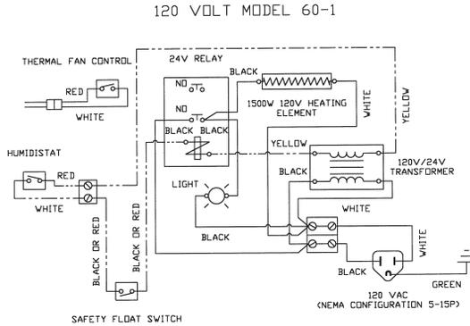
Figure 5 - Wiring diagram for Model 60-1 and F60-1 (120 volt) Steam Humidifiers.
