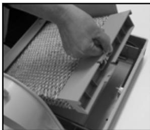
4. Wash all plastic and metal parts (except electrical parts and components) in humidifier cleaner or a 50 percent solution of vinegar and water.
