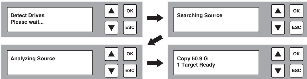
3. During the copy process the HDD Copy Cruiser IDE/SATA High-Speed will display progress information.
