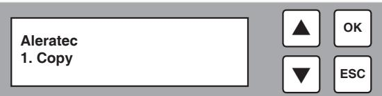
**Note:** Before copying be sure that the capacity of the target HDD is equal to or larger than the source hard drive.
