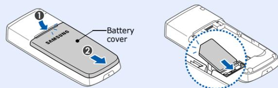
2. Install the battery and reattach the cover.
