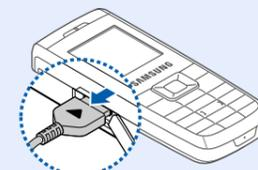
**Note:** Do not remove the battery from the phone without unplugging the adapter first. Otherwise, the phone may be damaged.
